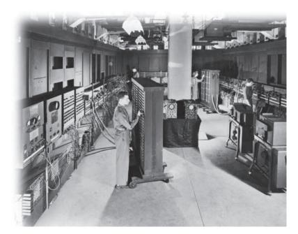
From this 1946 photo, you can see how computers have changed. This is the ENIAC, the world's first computer, which weighed 30 tons, was 8 feet high, 3 feet deep, and 100 feet long. Most cell phones have more computing power than this monstrosity.
