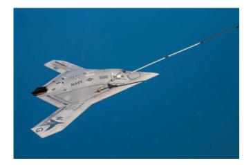
This pilotless drone, the Navy's X-47B, is being refueled in midair from a tanker plane.
